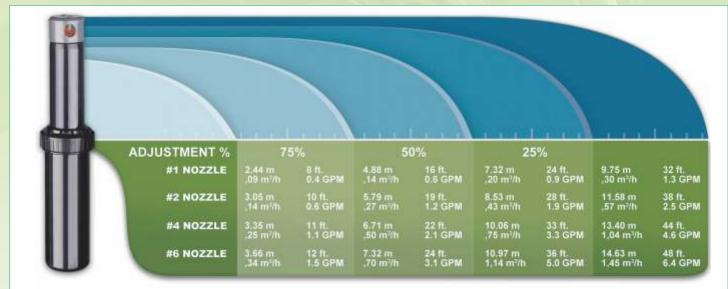
"With FLOW SHUT OFF mechanism. Radius reduction can be done up to 75% (No other pop up in the world has this feature). Pattern of spray remain undistorted in case of radius reduction."
